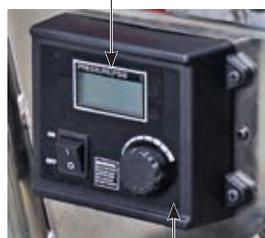
Control System includes Auto Stop Function when paint is used up
